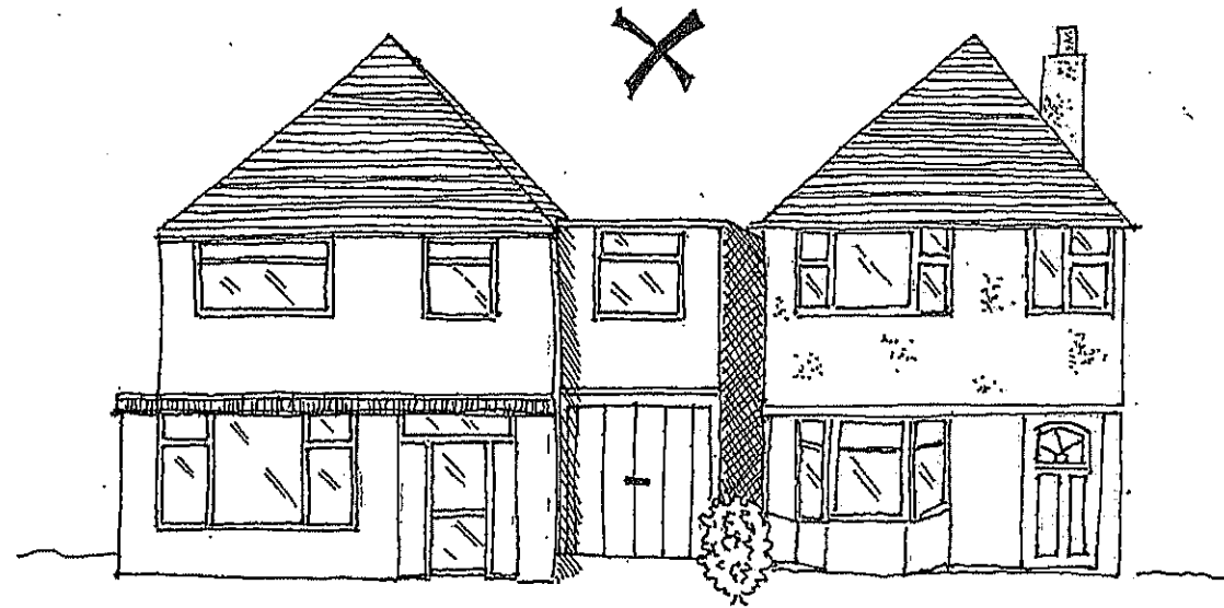
Fig. 5 -Unacceptable flat roof extension
