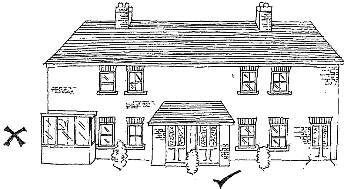
Fig. 9 -Single storey extensions to the front
